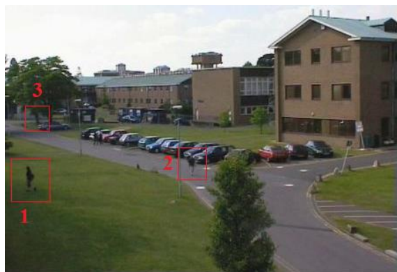
Figure 5: Example detections, PETS2001 dataset. (1) and (2) are true positives; (3) is a false positive.
