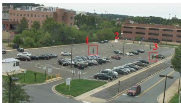
Figure 7: Example detections, VIRAT dataset. (1) is a true positive; (2) is a false negative; (3) is a false positive.
