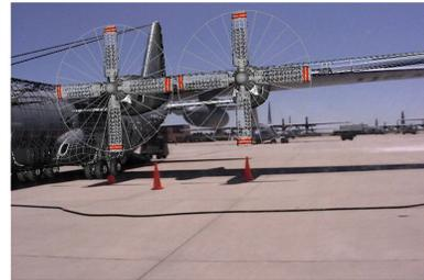
Figure 1: C-130 with cone fiducial targets and virtual overlays.
