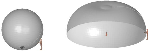
Figure 2: “Working volumes” for planar target (left) and cone target (right).
