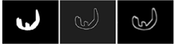
Fig. 7. Predicted rendered image of the femoral model (left) and its silhouette (center). The right image shows an expanded version of the silhouette where pixels are encoded with their closeness to the contour (within a small band).
