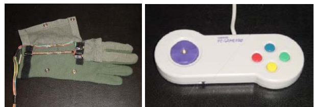
Figure 2 Alternative input devices: data glove (left) and game pad (right).
