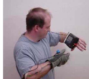
Figure 1 User interface with wrist-mounted display and data glove.
