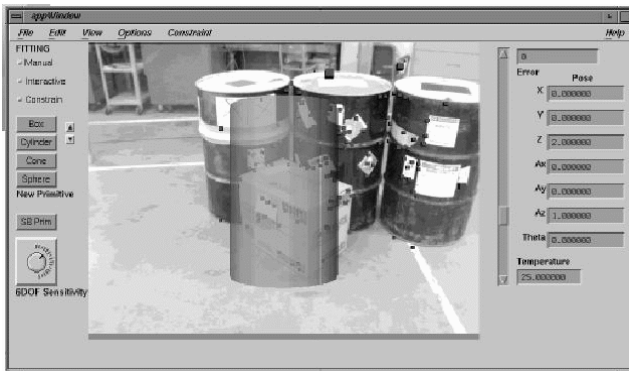
Figure 3 User interface for model fitting application, showing cylinder model in initial pose.
