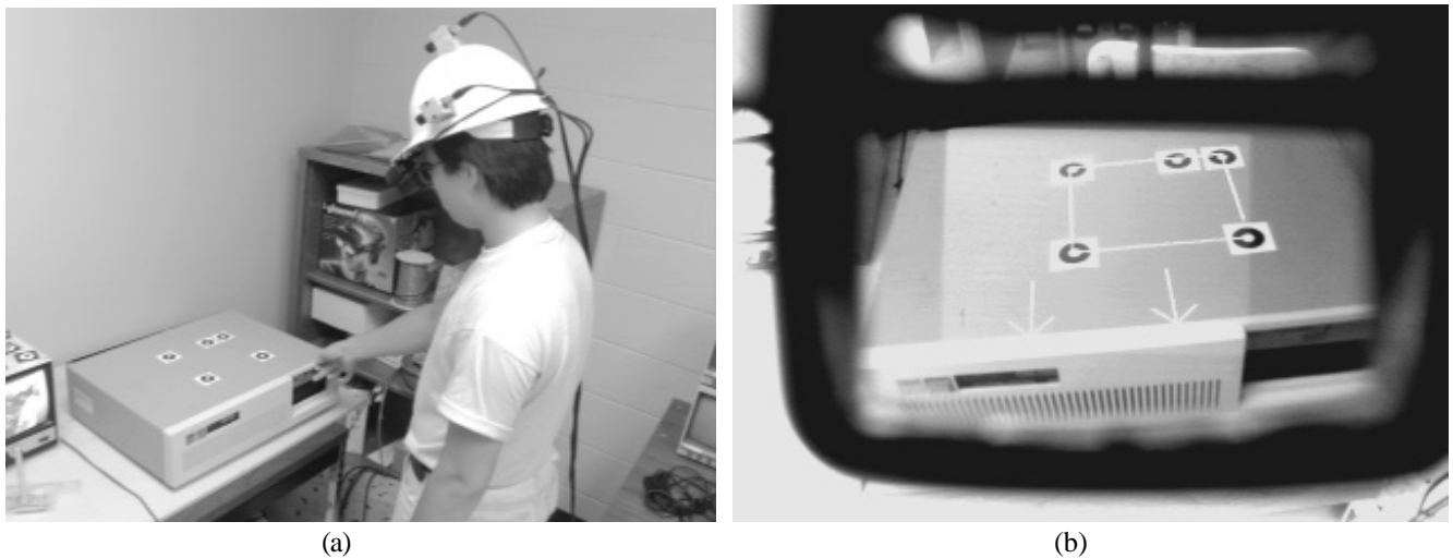
Figure 7 (a) Person wearing AR system. (b) View through head-mounted display, showing overlays indicating direction to remove cover of PC.
